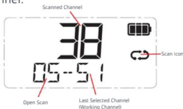
**NOTE:** If there are less than two channels programmed into the Scan memory when you press the **SCAN** key, an error beep will be heard and **SCANERROR** will be displayed.
