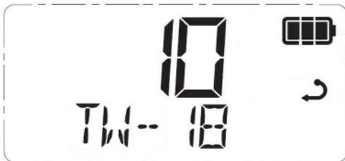
**NOTE:** When Triple Watch is active, you can change the selected channel at any time by rotating the **Channel Selector** knob or pressing the **▲▼** keys. Your radio will continue to monitor your two Priority Channels as well as your newly selected channel.
