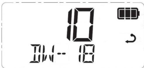
**NOTE:** When Dual Watch is active, you can change the selected channel at any time by rotating the **Channel Selector** knob or pressing the ▲ ▼ keys. Your radio will continue to monitor the last selected **Priority Channel** and your newly selected channel.
