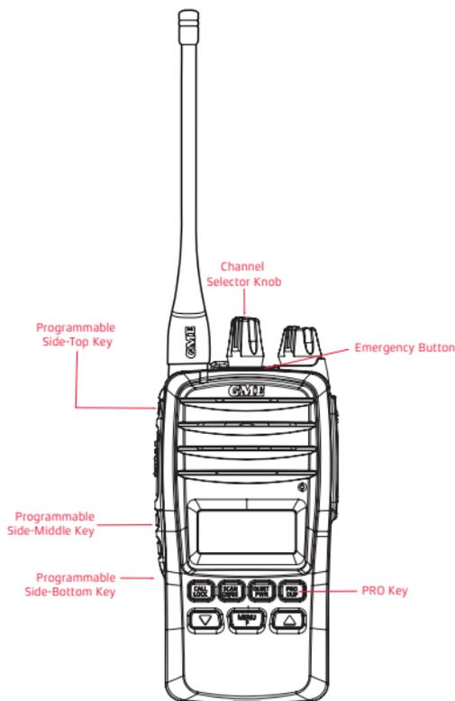
**Programmable Side Keys:** These keys can be programmed with up to 3 separate functions each. (press / hold / Menu Key then press).
