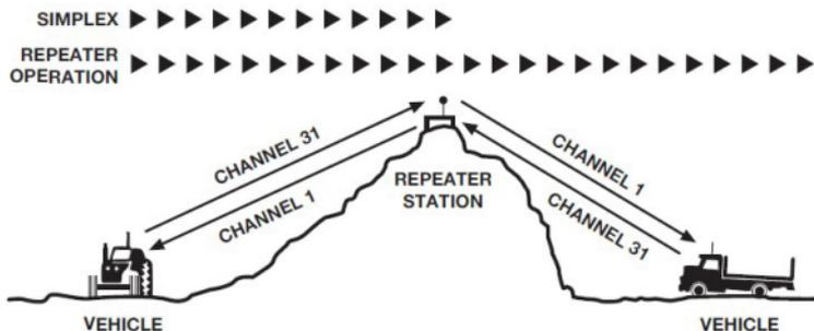
The Duplex function operates only on designated repeater channels. These are channels 1–8 and 41–48. When Duplex is enabled on one of these channels, the CP30 will receive on the selected channel but will transmit 30 channels higher. i.e. if channel 1 is selected the CP30 will receive on channel 1 but transmit on channel 31.
